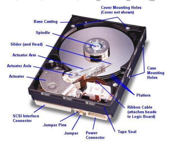
Hard disk drives are almost as amazing as microprocessors in terms of the technology they use and how much progress they have made in terms of capacity, speed, and price in the last 20 years. The first PC hard disks had a capacity of 10 megabytes and a cost of over \$100 per MB. Modern hard disks have capacities approaching 100 gigabytes and a cost of less than 1 cent per MB! This represents an improvement of
